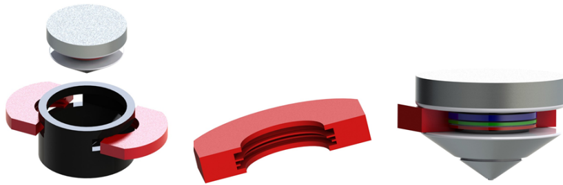
Figure 9: Berthing mechanism for hub/cartridge mating
