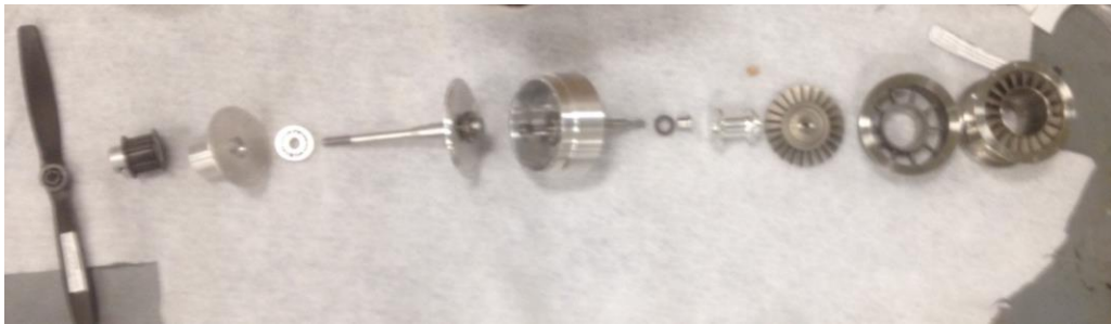
Figure 7: Turboprop add-on parts layout before assembly in the correct order
