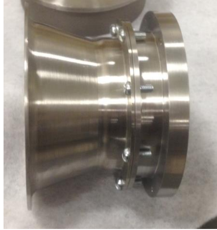
Figure 6: Picture of interstage nozzle guide vanes on the left attached to the coupler in the right
