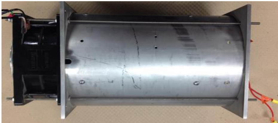
Figure 5: 8Ω load cell to drive electrical circuit current to 3A.
