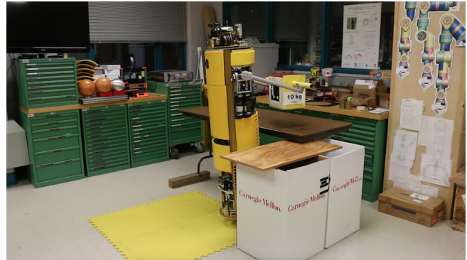
Fig. 8. The ballbot is transporting a 10 kg heavy object from A to B.
