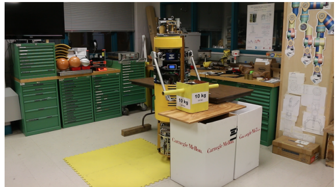
Fig. 9. The ballbot successfully placed the object on the table.
