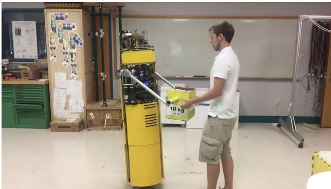
Fig. 7. The ballbot delivers a 10 kg heavy object to a person
