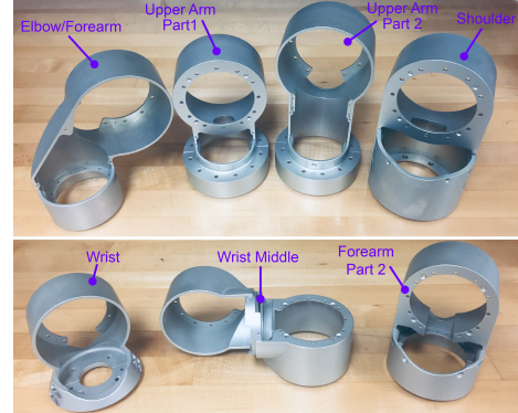
Fig. 10: Exoskeleton shell structural links. Each link is machined from a single block of 7075 aluminum using 5-axis milling.
